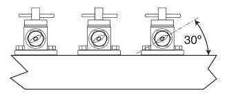
Figure 8. Adjusting the Spray Bar Nozzles.
