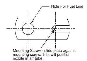
Figure 28. Electrode Assembly Installation
