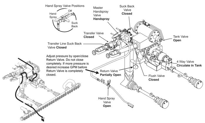
Figure 17. Valve Positions for Handspray.
