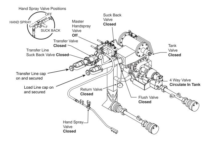
Figure 11. Valve Positions for Loading Through the Manhole.
