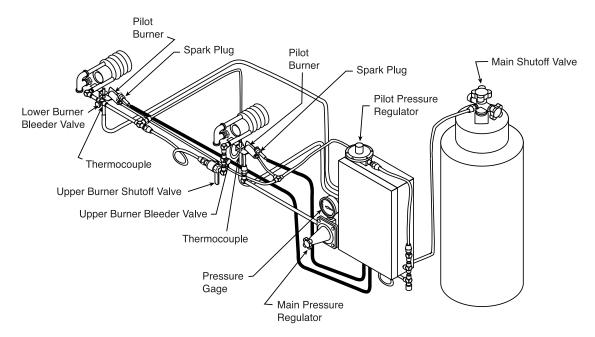
Figure 25. Burner System with Auto Ignition and Temperature Control.
