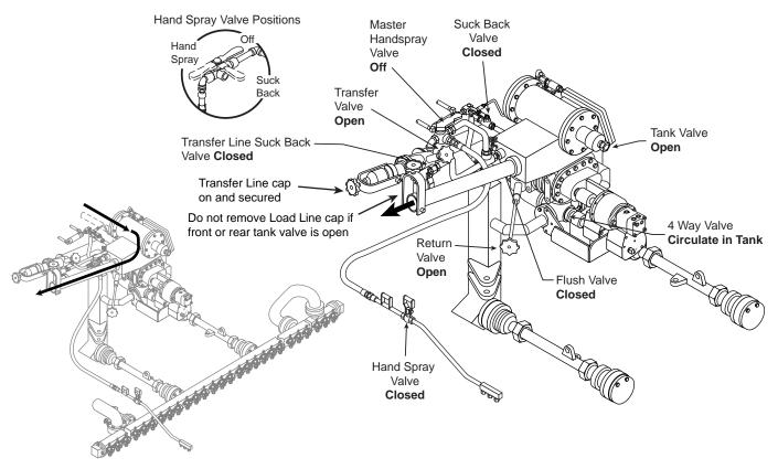
Figure 20. Valve Positions for Unload with External Pump.
