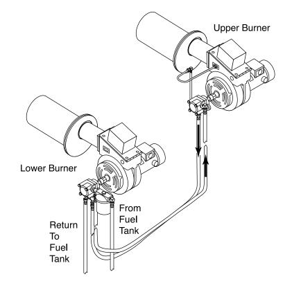
Figure 26. Electric Burner System.
