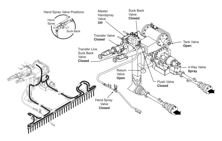
Figure 16. Valve Positions for Spraying Through the Bar.
