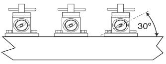
Figure 31. Nozzle Angle Adjustment.
