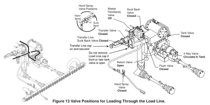
A pump rate of 100 GPM is recommended to begin the loading operation. The pump rate can be increased at any time after loading has begun. Depending on material viscosity, as the loading rate is increased, the asphalt pump may cavitate. When this happens, the pump will make a distinctive sound, easily recognized with experience. Short periods of operation while the pump is cavitating will not damage the pump but you should not operate the pump in this condition for extended periods.
