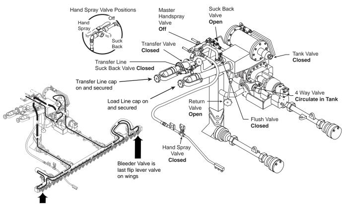
Figure 18. Valve Positions for Spray Bar Suck Back.
