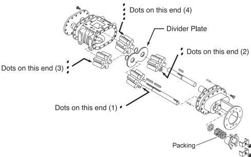
Figure 33. Etnyre Asphalt Pump.
