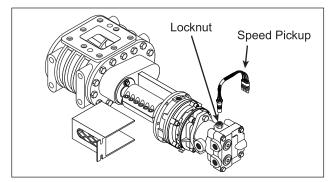
Figure 30. Hydraulic Motor.
