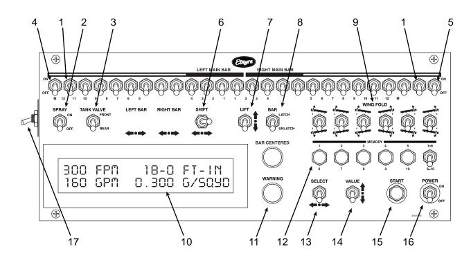
Figure 6. Cab Control Panel Components.
