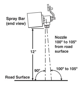
Figure 32. Nozzle Height Adjustment.
