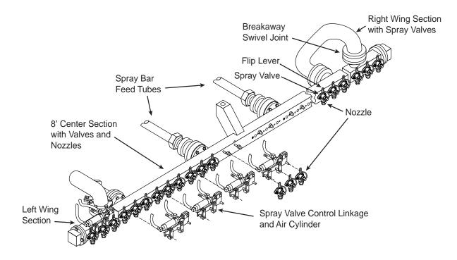
Figure 4. Spray Bar Component Identification.
