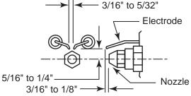
Figure 27. Burner Electrode Adjustments.
