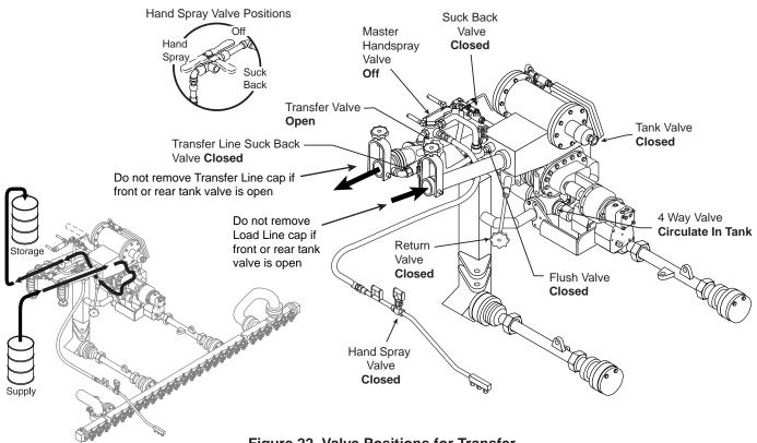
Figure 22. Valve Positions for Transfer.
