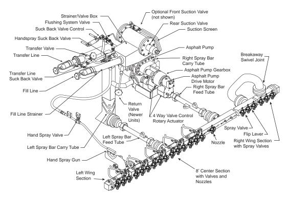
Figure 3. Rear Component Identification.
