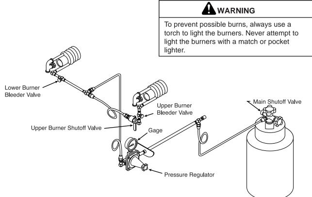
Figure 23. Manual Control Burner System.
