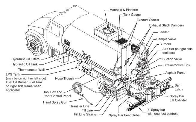
Figure 2. Rear and Side Component Identification.
