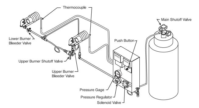
Figure 24. Outfire Controlled Burner System.
