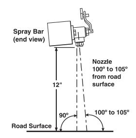
Figure 9. Adjusting the Spray Bar Height.
