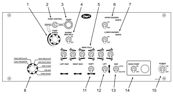
Figure 7. Rear Control Panel Components.
