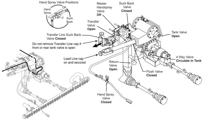
Figure 21. Valve Positions for Unload withDistributor Pump.
