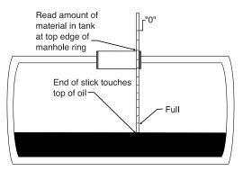
Figure 12. Using the Measuring Stick.
