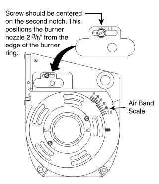
Figure 29. Nozzle Adjustment.
