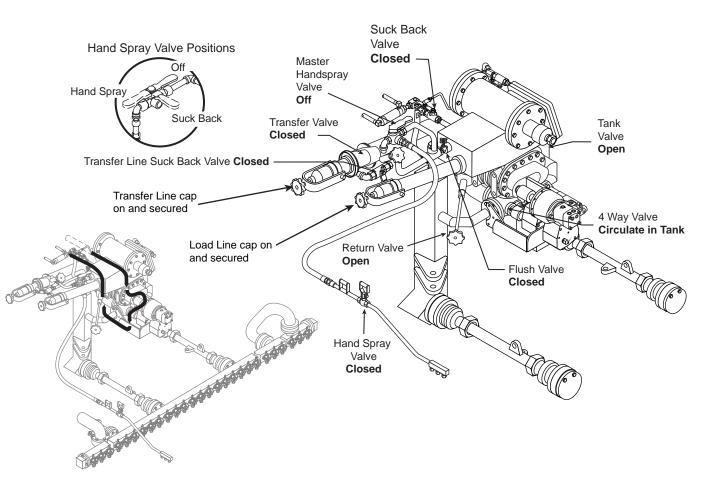
Figure 14. Valve Positions for Circulating in the Tank.
