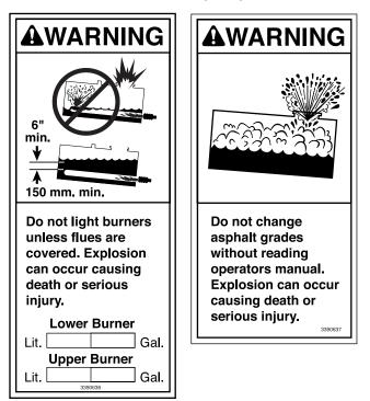
Use the measuring stick as shown in Figure 9 in the *Using the Measuring Stick* section to determine the amount of product in the tank before lighting burners. The minimum amounts shown on the warning placard only apply if the tank is level.
