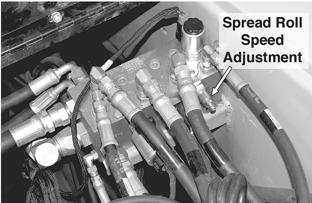
Figure 30. Conveyor/Auger/Spreadroll Manifold Spreadroll Flow Control Valve
